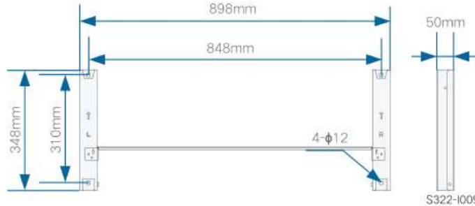
Figure 4-1 Dimensions of Mounting-bracket
